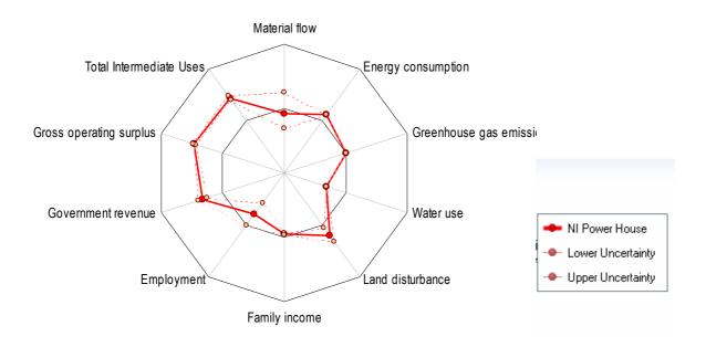
Fig. 13: Benchmark spider diagram for the power house (red bold polygon, BL<sup>3</sup> output). The central polygon represents the Australian economy-wide average performance. The centre locates ten-times-*better* performance (*not* ten-times-lower), the outer rim ten-times-*worse* performance (*not* ten-times-higher). Environmental indicators are compared per-kWh<sub>el</sub> generated, with the remaining social and economic indicators per \$ of output as usual.
