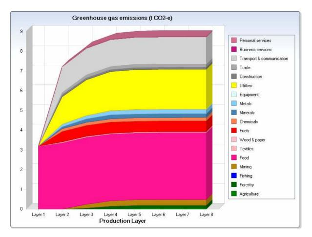
Fig. 6: Production Layer Decomposition of greenhouse gas emissions for Cascade soft drinks (BL<sup>3</sup> output). Layer 1 represent Cascade, layer 2 Cascade's suppliers, layer 3 the suppliers of Cascade's suppliers, and so on. The colours reflect a rough grouping of industry sectors in the Australian economy.
