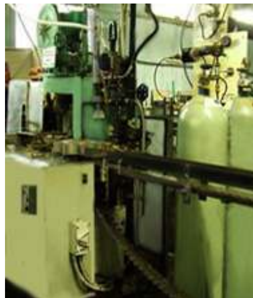
Fig. 3: Bottling line and CO 2 for carbonisation of soft drinks.
